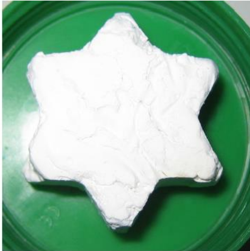
Fig. 4. Aerogel monoliths take the shape of the mold where the gel is prepared: starch aerogel obtained by supercritical drying from a hydrogel prepared in a mold for Christmas cookies.
